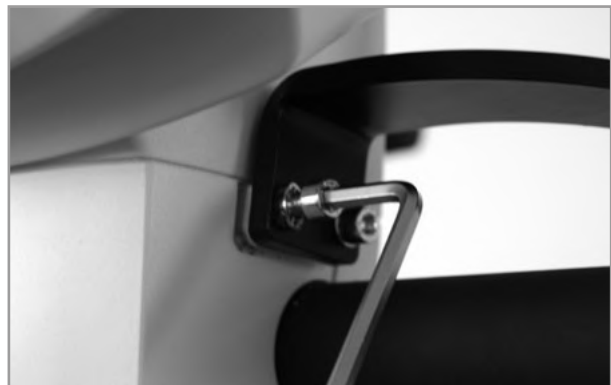
Figure 4-7: Mounting the leadwire holder
