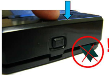
Figure 15: NR-1207-E / NR-1207-3 battery installation
